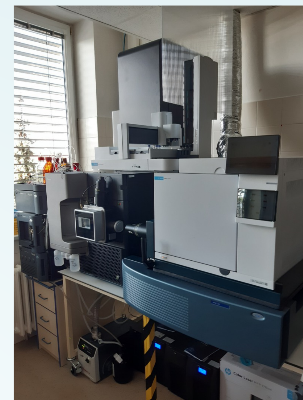
Fig. 2: High resolution Waters Xevo G3 QToF coupled with gas chromatograph Agilent 8890A via APGC interface and UHPLC Waters Acquity acquired with financial support of The State Environmental Fund of the Czech Republic, as the Programme Operator of the Programme „Environment, Ecosystems and Climate Change“, supported by the Norway Grants 2014–2021. System will be used for pesticide and pharmaceutical screening, confirmation of potential interferences and untarget screening of new emerging contaminants.
