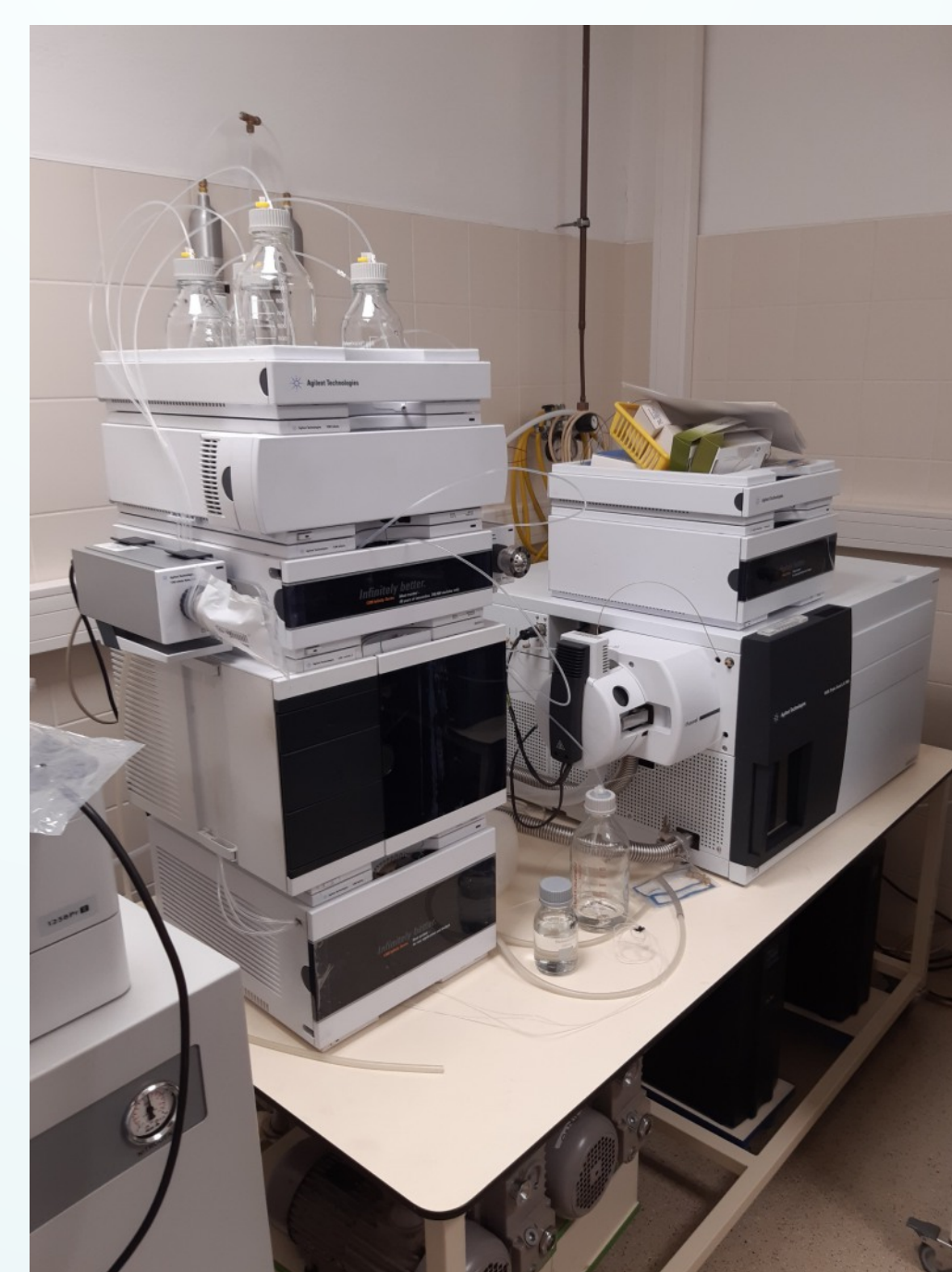
Fig. 4: Agilent Technologies Triple Quad 6495A coupled with UHPLC 1290 used for multiresidue analyses of pesticides, their metabolites, pharmaceuticals and perfluorinated alkyl substances in surface waters measured in negative ionization mode.
