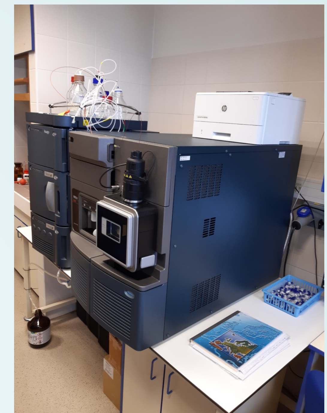
Fig. 3: Waters Triple Quad XEVO TQ-XS coupled with UHPLC Acquity used for multiresidue analyses of pesticides, their metabolites and pharmaceuticals in surface waters measured in positive ionization mode.
