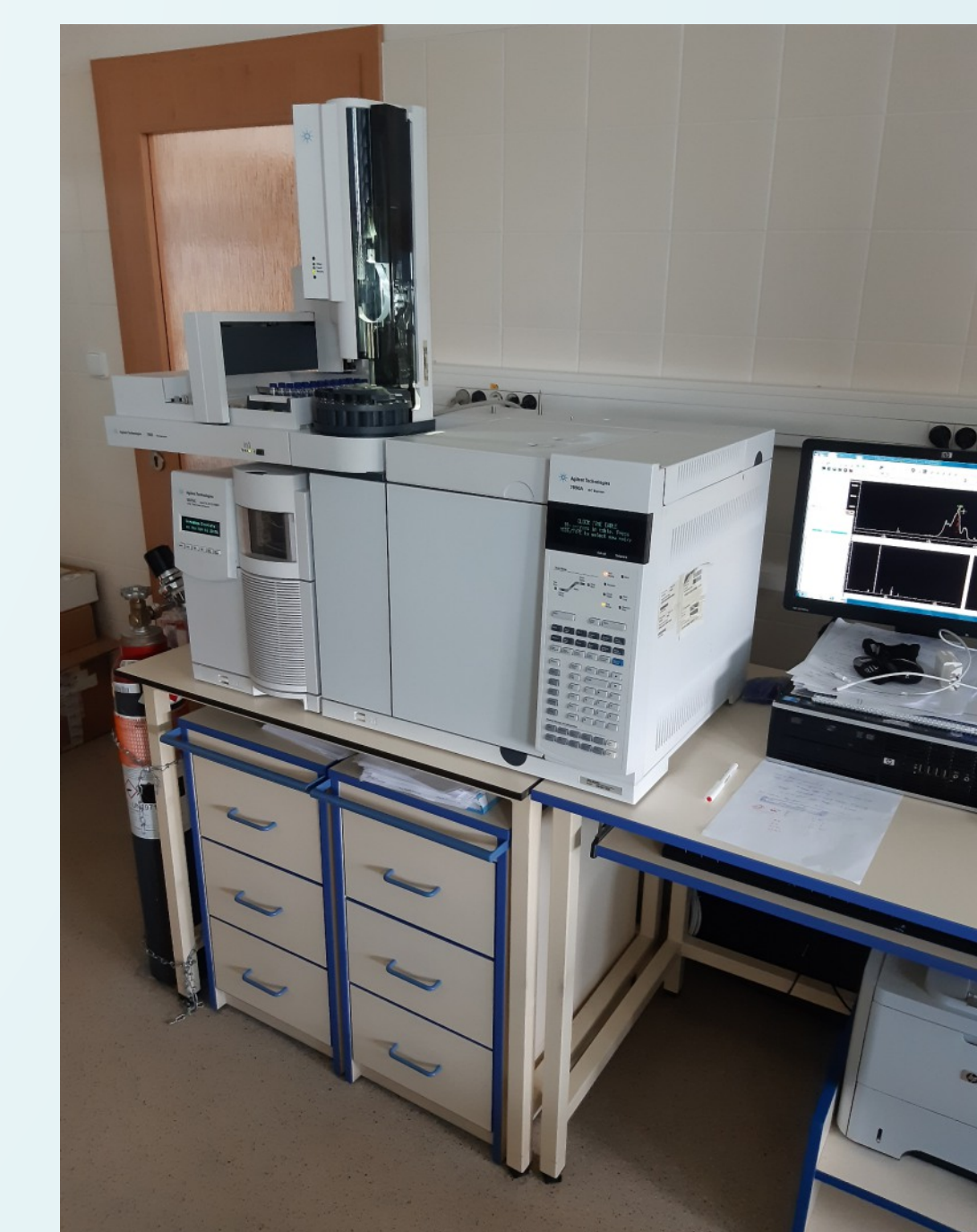
Fig. 6: Agilent Technologies Single Quad GC-MS 5975C EI/CI (negative chemical ionization) coupled with gas chromatograph 7890A used for measurement of chlorinated paraffins, pyrethroids (cypermethrin), PBDEs in solid matrices and waters.
