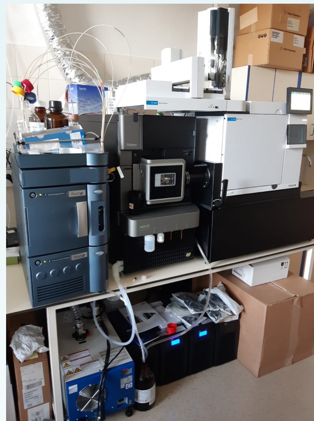
Fig. 1: The New Chromatographic Mass Spectrometric System consisting of Triple Quad Waters XEVO TQ Absolute coupled with gas chromatographs Agilent 8890A via APGC interface and UHPLC Waters Acquity acquired with financial support of The State Environmental Fund of the Czech Republic, as the Programme Operator of the Programme „Environment, Ecosystems and Climate Change“, supported by the Norway Grants 2014–2021. System will be used for ultrasensitive analyses of selected water pollutants: Polyfluorinated Alkyl Compounds (PFACs), pharmaceuticals, hormones, pesticides, etc.
